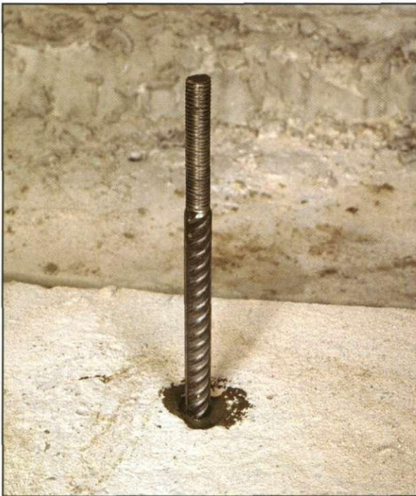
Figure 14 Concrete failure possibly due to shallow fixing depth or cracking to concrete. This is an unreinforced slab.
