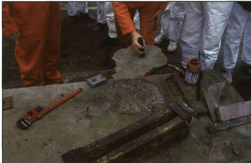
Figure 14 Concrete failure possibly due to shallow fixing depth or cracking to concrete. This is an unreinforced slab.
